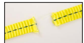
Failure due to sharp edge conditions
