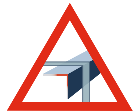
Global Sharp Edge Symbol Radius as sharp as .005 in. (.13mm)
